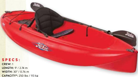
FITTED HULL WEIGHT\*: 46 lbs / 21 kg FULLY RIGGED WEIGHT\*: 50.5 lbs / 23 kg **HULL CONSTRUCTION:** Rotomolded Polyethylene
